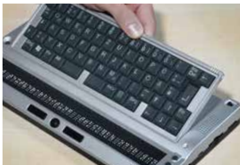
Switching the input between braille and a standard keyboard simply by exchanging the keyboard module.
