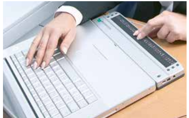
SuperVario2 can be combined as a braille display with PC, MAC and notebook.
