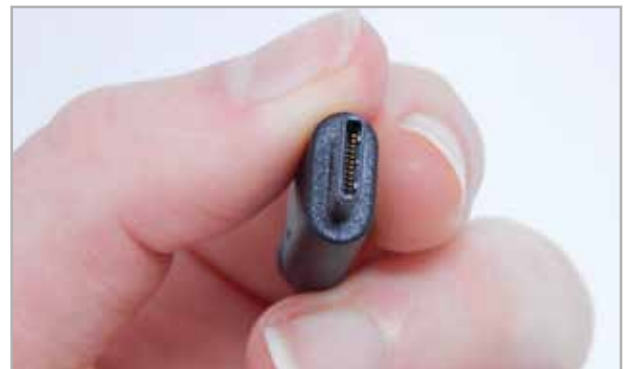
The USB Type C connector can be inserted into Vario 340 in either direction.
